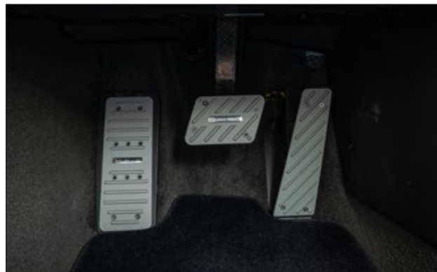
Sport pedals ..... BX7 367 127 3 parts, acceleration, brake, foot rest
