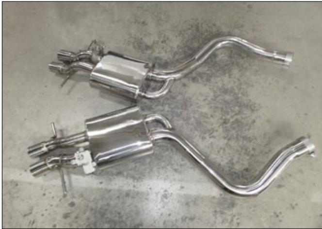
Mufflers 223 221 009 set - left & right with throttle control
