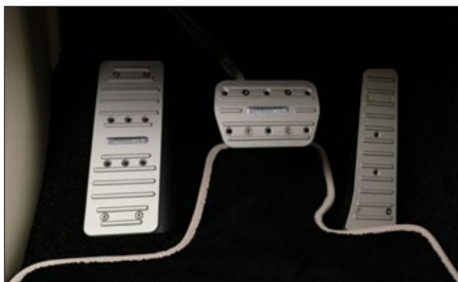
Sport pedals ..... LRR 367 127 3 parts, acceleration, brake, footrests
