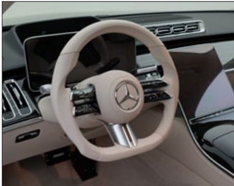
Sport steering wheel ..... 223 351 411 leather, color selectable (C) modification only, OE-part required
