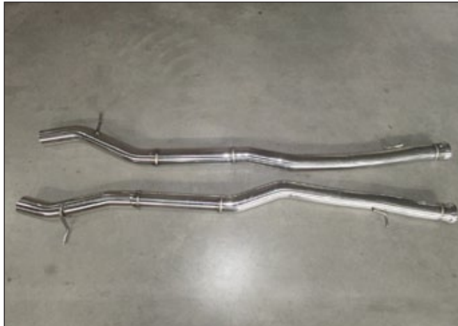
Exhaust middle pipes 22M 221 139
