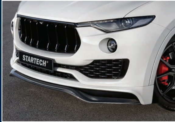
M156-200-30 Fronteinsatzelement, PUR R-RIM, inkl. Carbon Frontflügel Front bumper insert, PUR R-RIM, incl. carbon front wing
