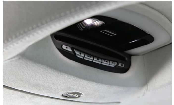
Bedienelement der Dachhimmel-Mediakonsole Operation control unit of the roof mounted media console
